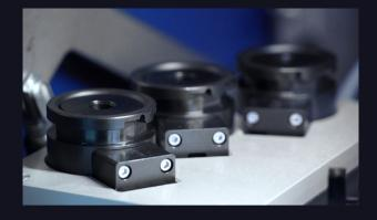
The Module DERIVATIZATION features three spraying nozzles generating different droplet sizes to suit the properties of the selected reagent.
