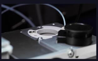
The cleaning station washes the nozzle from the inside and the outside. Meanwhile, the HPTLC plate is moved to the subsequent heating step.
