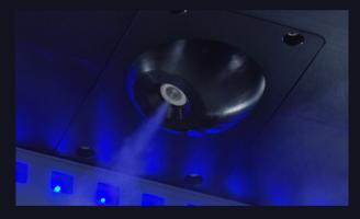
Employing the patented micro-droplet spraying technology, the reagent spraying nozzles generate an extremely fine reagent mist, which evenly distributes in the derivatization chamber and gradually settles down on the plate.
