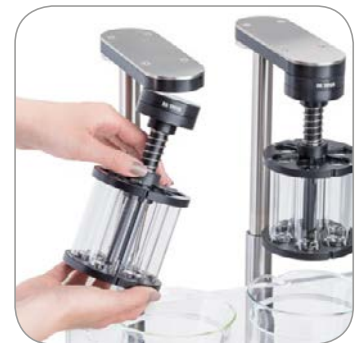
Simple & practical: the testing baskets are magnetically coupled
