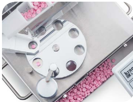
Fast, precise weighing of tablets or capsules with the automatic CIW weighing system
