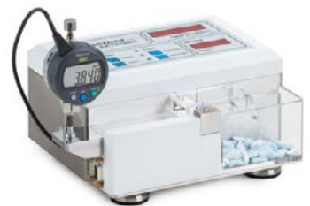
HC 6.2 with external thickness gauge and scale
